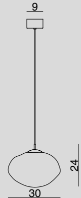
GIG1653.1L SOSPENSIONE A ROSONE / HANGING LAMP WITH CANOPY Glass 1 x Ø 30 cm - Cable 200 cm 1 x LED 8,4 W DIMM
