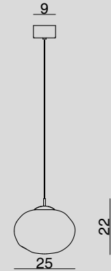
1643.1L SOSPENSIONE A ROSONE / HANGING LAMP WITH CANOPY Glass 1 x Ø 25 cm - Cable 200 cm 1 x LED 6 W DIMM
