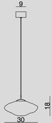
1663.1L SOSPENSIONE A ROSONE / HANGING LAMP WITH CANOPY Glass 1 x Ø 30 cm - Cable 200 cm 1 x LED 6 W DIMM
