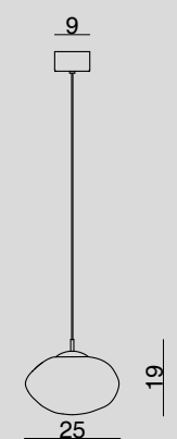
1653.1L SOSPENSIONE A ROSONE / HANGING LAMP WITH CANOPY Glass 1 x Ø 25 cm 1 x LED 6 W DIMM
