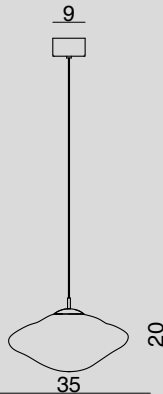
GIG1663.1L SOSPENSIONE A ROSONE / HANGING LAMP WITH CANOPY Glass 1 x Ø 35 cm - Cable 200 cm 1 x LED 8,4 W DIMM
